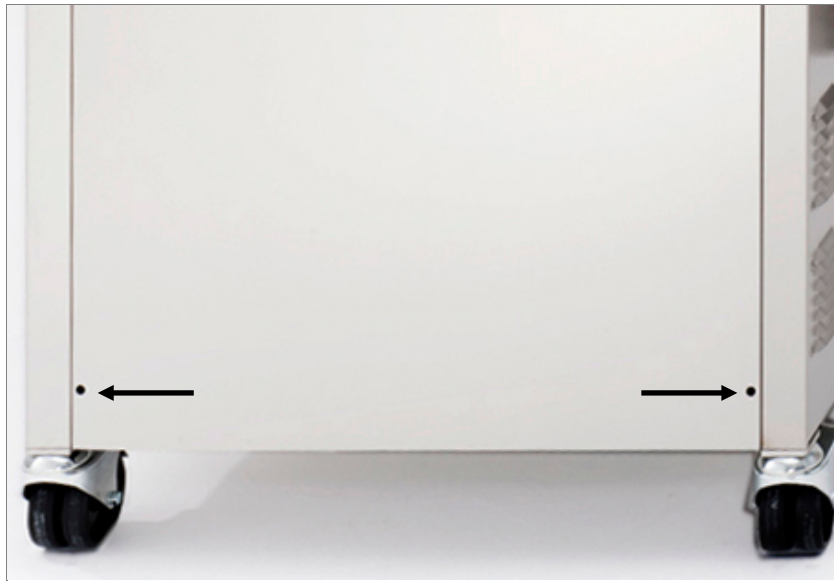
Fig. 9.5.1. Position of the 2 Allen screws
