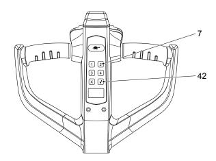
The truck can only be started with the correct access code.
