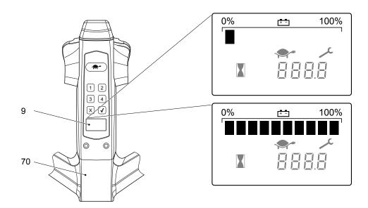
The charge status indicator of the battery is integrated in the display unit (9) on the tiller head (70).
