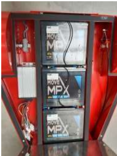
Chassis interior with batteries, control unit and cable to safety foot switch
