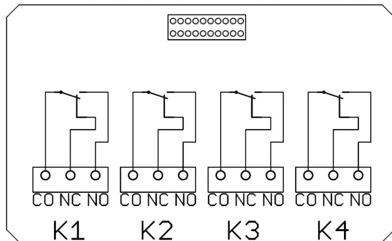
The connection diagram shows the relay module in de-energized state.
