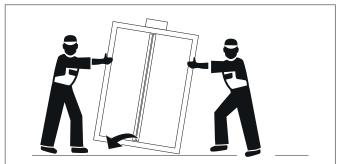
After installing the cabinet, remove the protections for transport present along the door joints.
