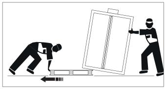
After removing the pallet, lower the cabinet slowly and without jolts to avoid damaging it.
