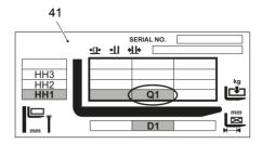
The capacity plate (41) indicates the maximum capacity Q (in kg) for a given load centre distance D (in mm) and corresponding lift height H (in mm) for the truck with a horizontal load.
