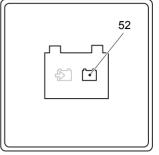
If the LED is lit red, load can no longer be lifted. Lifting is only enabled when the battery connected is at least 70% charged.
