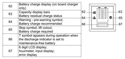
In addition, service messages for the electronic components and parameter changes are displayed.
