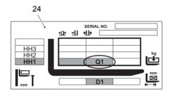
The capacity plate (24) indicates the maximum capacity Q (in kg) for a given load centre distance D (in mm) and corresponding lift height H (in mm) for the truck when raising a load.
