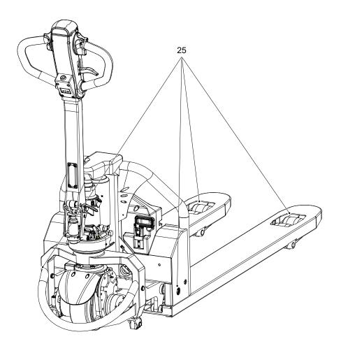
The strap points (25) under the frame and at the fork tips are intended for lifting the truck with crane lifting gear.
