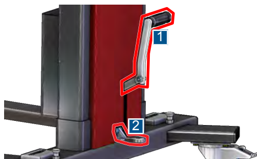
Fig. 35: Lifting and lowering
