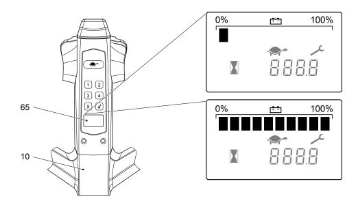
The charge status indicator of the battery is integrated in the display unit (65) on the tiller (10).
