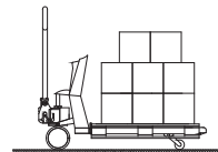
Correct lifting of load
