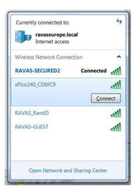
Step 2: connect to the xPico240\_CD0FC9 (last six digits depend on the address of the Xpico installed). By default the SoftAP mode is enabled with a default SSID of xPico240\_xxxxxx. Where xxxxxx are the last six characters of the unique xPico 240 serial number. This number is available on the module label. For example if the serial number on label were 0080A54E7F then the SSID would be Xpico240\_A54E7F.
