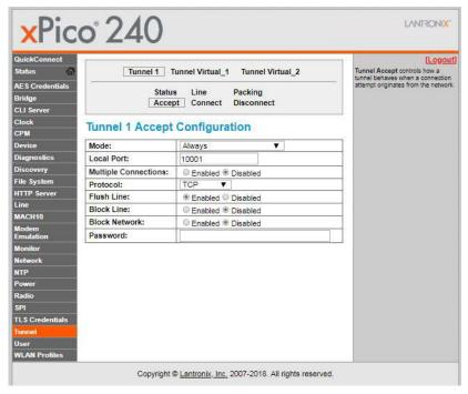
In 'Tunnel'/ 'Accept' set 'Flush Line' to Enable this can be useful when operating in a busy area where many devices share the same Access Point.
