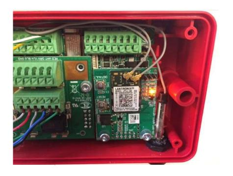
TIP when needed – you can use the <u>default button for</u> a total reset of the unit (press and hold for more than 6 s.)
