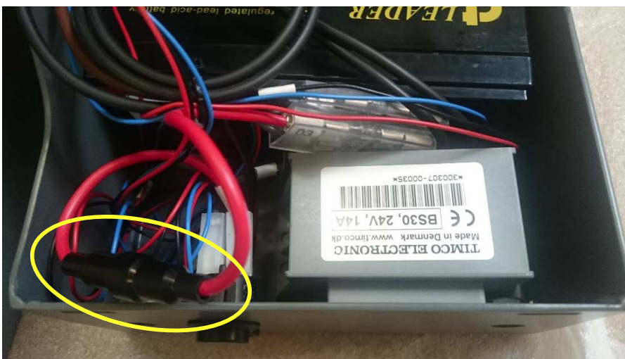
3. Open black fuse housing by unscrewing, to replace fuse
