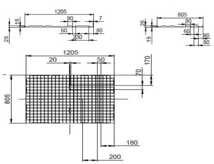
\*All load capacity data is only valid in case of evenly distributed load. For all indicated dimension tolerances of +/- 3 mm apply.
