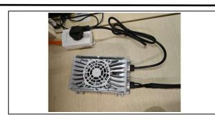
Using the charger output connector, connect the battery.
