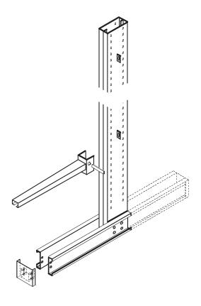
The load labels shall be attached to the columns where they will be clearly visible. If the row consist of all the same parts, one label will be placed on the first and one on the last column, and maximum one on every third column in between.
