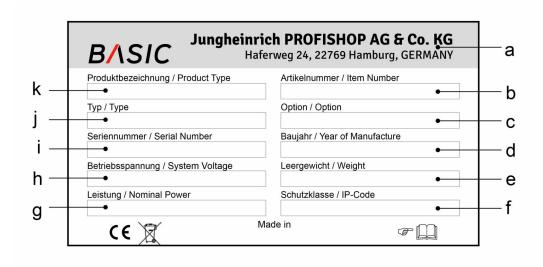
Fig. 1: Data plate (schematic)
