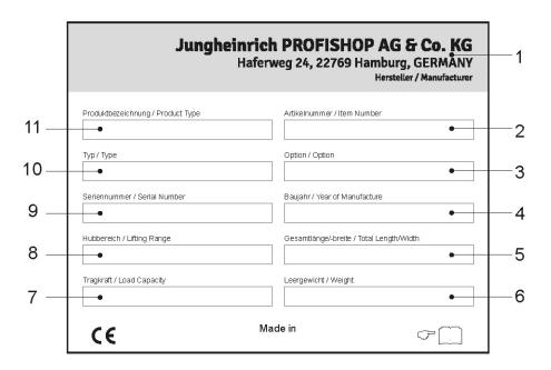
Fig. 1: Data plate (schematic)
