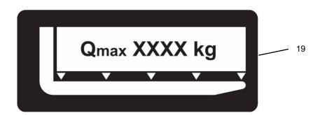
The capacity plate (19) indicates the maximum capacity Q (in kg) for a given load centre C (in mm).
